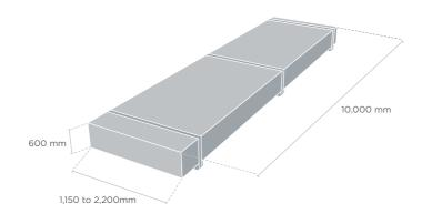
EGA billets are produced using Airslip technology and are ultrasound inspected and homogenised before delivery. A large proportion of our annual production is cast in high extrudability 6063 alloy. These products are used for construction (windows and door frames), transportation, engineering, consumer durables, automotives, forging, as well as many other applications.
