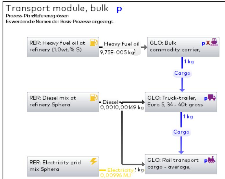
**Figure 7: adjustable IAI transport module model for raw material transport**
