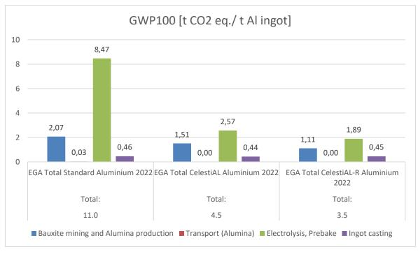
Figure 35: GWP results of EGA Total Aluminium products in comparison
