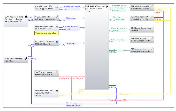
Figure 8: ATS anode production model for AT Standard Aluminium
