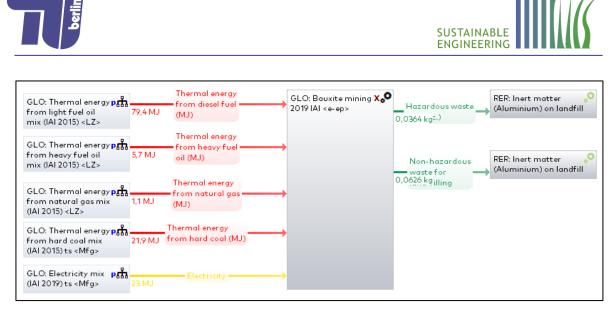
Figure 5: Bauxite mining model based on IAI GLO 2019 data
