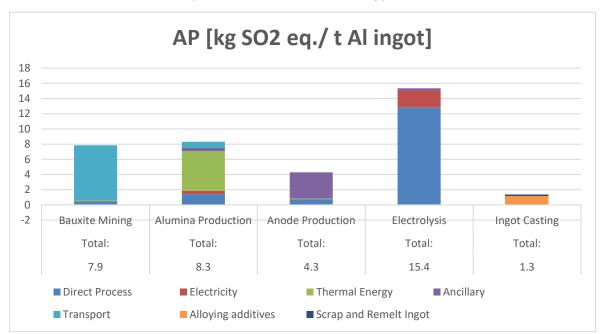
Figure 18: EGA Total Standard Aluminium process contributions in AP
