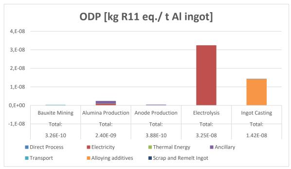
Figure 23: EGA Total Standard Aluminium process contributions in ODP
