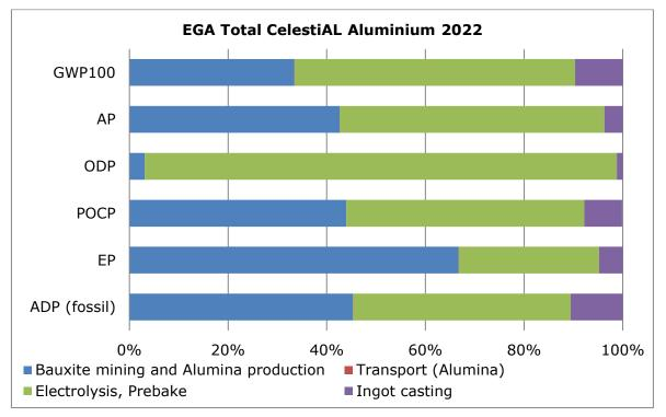
Figure 27: Overall LCIA profile of EGA Total CelestiAL Aluminium
