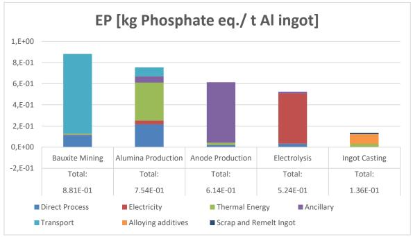
Figure 19: EGA Total Standard Aluminium process contributions in EP
