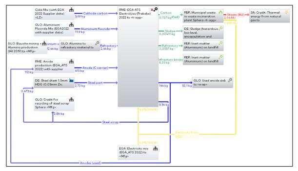
Figure 9: Electrolysis model for EGA ATS
