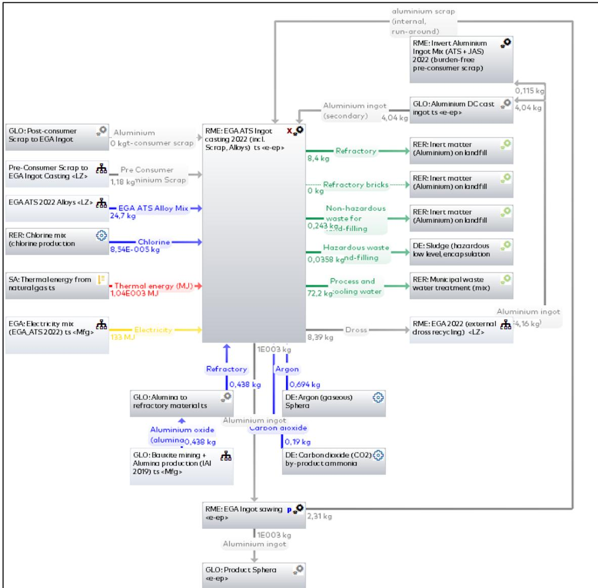
Figure 10: Ingot casting model for EGA ATS
