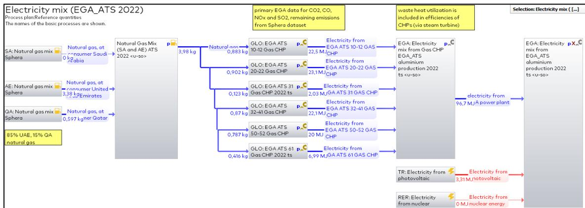
**Figure 4: Electricity mix model for EGA ATS site**
