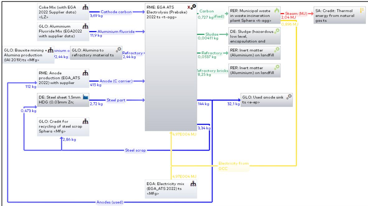
**Figure 9: Electrolysis model for EGA ATS**
